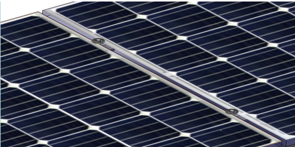
Insert Bolts into the threaded PEM Nuts in the top of each bracket as shown and tighten to 65 in-lb.
