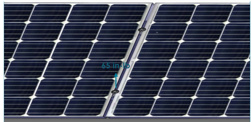
Place PV Module on brackets and line Grounding End Plate up to span both brackets.
